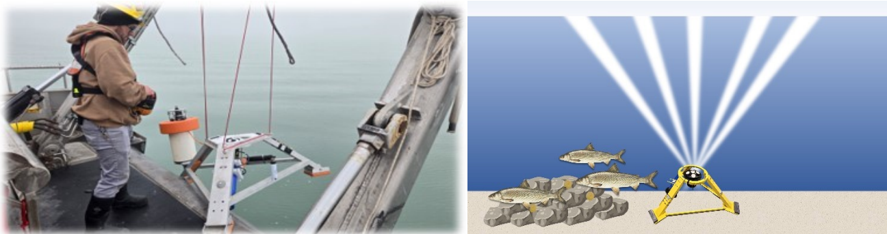
Figure 1. The left image shows the monitoring station being deployed to investigate the influence of ice cover on the Niagara Reef. The right image is a rendering of the monitoring station deployed near a fish spawning reef.
